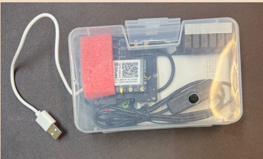
Data Broker, consisting of a Raspberry Pi Zero W with a Notecard Pi hat, a power cable and power button, a 10000-mAh power bank and a heat sink
