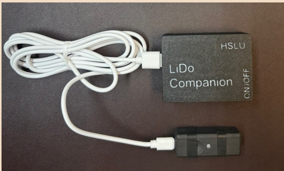
36 LiDo (bottom) and LiDo Companion (top) connected together with a two-meter long USB to micro-USB cable.
